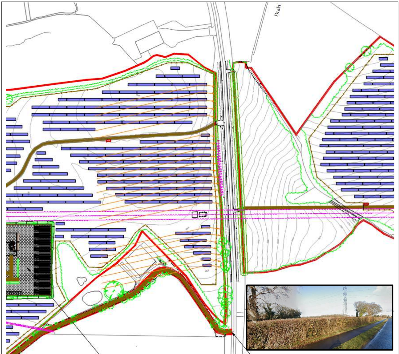
Fig 13 –Setting Sun Incident rays showing potential for glint in the direction of the A4226 but being caught by the existing hedgerow & trees (see inset).
